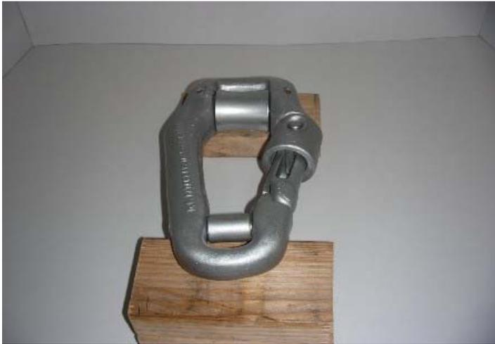
**STEP 1:** Clear a stable area. Using solid materials create 2 points of elevation. Place the Ring on top of these 2 points with the Push-Button facing upwards. Make sure the pivoting end of the Sleeve Assembly is free of the point of elevation so that the pin may be hammered out following grinding.
