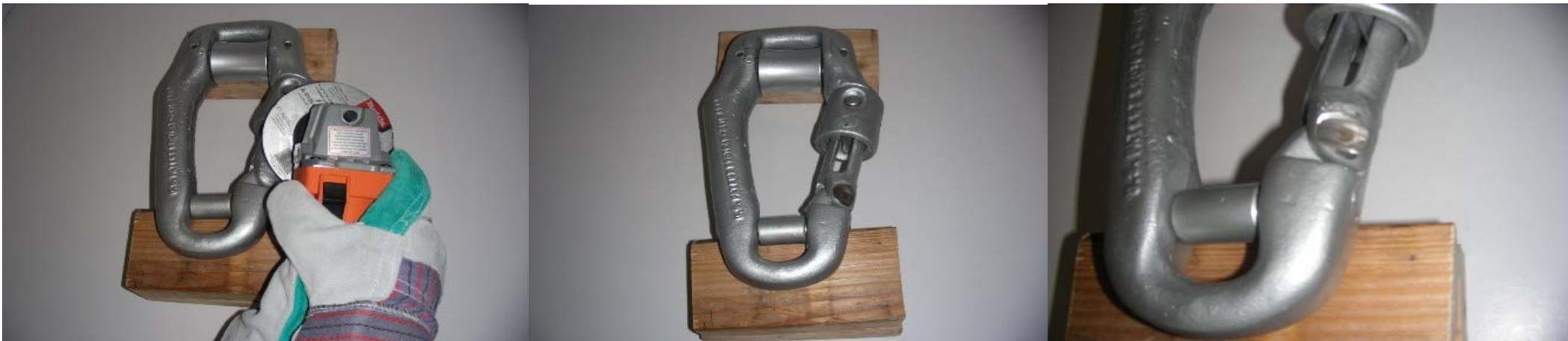
**STEP 2:** Using a grinder, grind away the welded area on the pivoting end of the Sleeve Assembly until the pin inside is visible.
