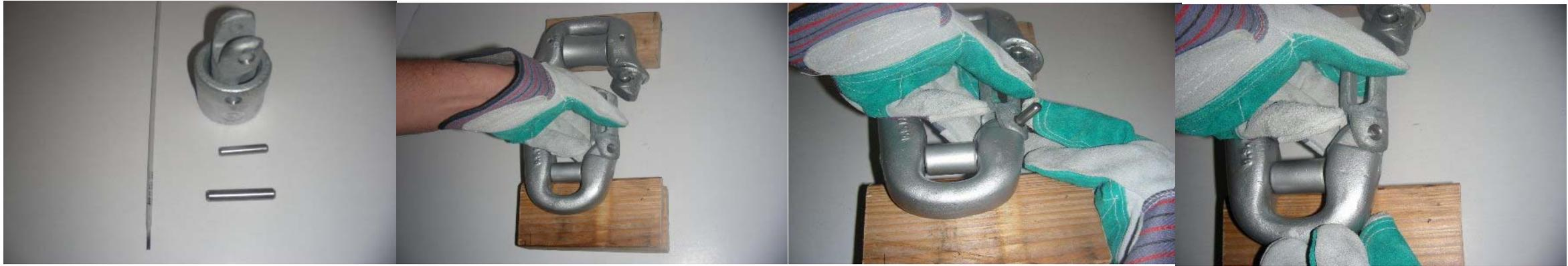
**STEP 5:** Place new Sleeve Assembly next to work area. Grasp only the pivoting end of the new Sleeve Assembly & line its' holes up with the holes for pin. Place the smaller pin into the hole. Be sure to block the other end of the hole so that the pin does not fall out.
