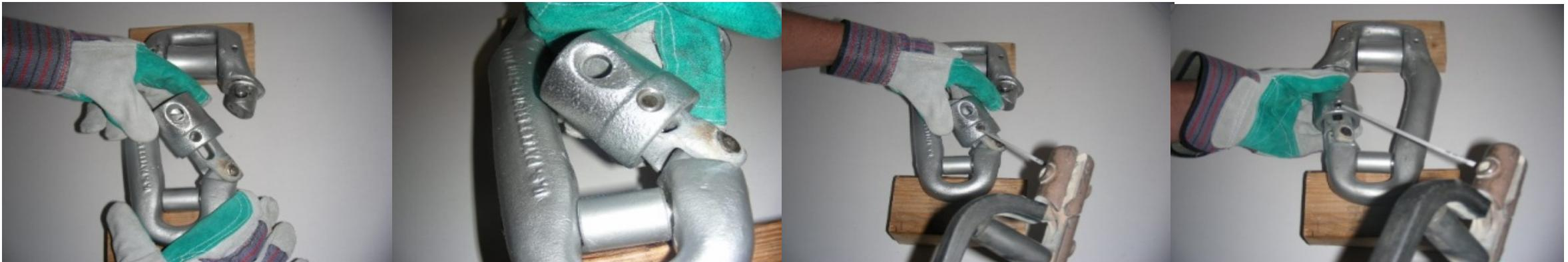
**STEP 8:** Now slide the sleeve piece of the new Sleeve Assembly onto the pivoting piece. Place the large pin into the hole. Be sure to block the other end of the hole so that the pin does not fall out. Using the stick of special welding rod provided, weld over the pin & hole. Once finished, flip the Ring over & repeat the process on the other side. Slide the Sleeve up & down to make sure the part operates properly.
