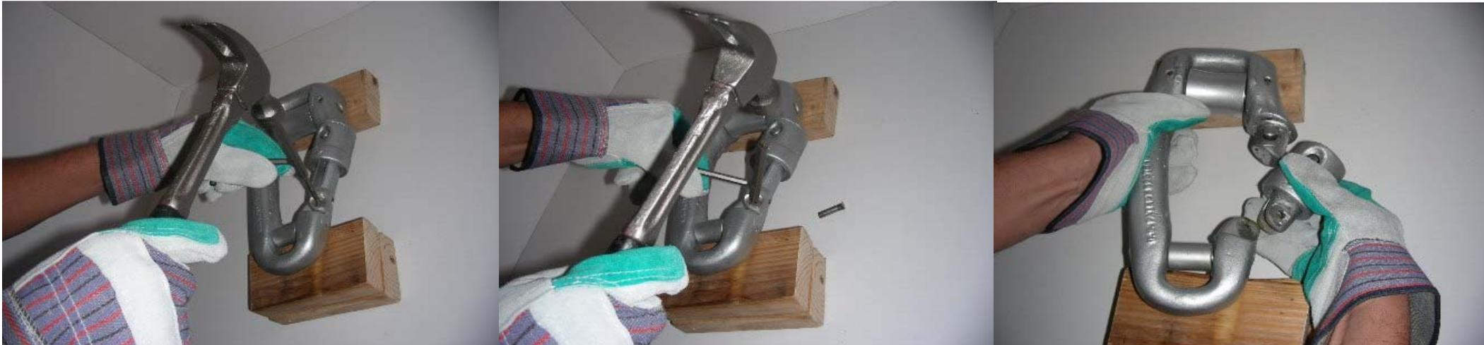
**STEP 4:** Grasp & flip the Ring over again so that the Push-Button is now facing upwards. Place the narrow end of the Tool Set over the now exposed pin. Hammer down on the opposite end of the Tool Set until the pin falls down & out of the Ring. While grasping the Sleeve Assembly push down on the Push-Button & remove the Sleeve Assembly from the Ring.
