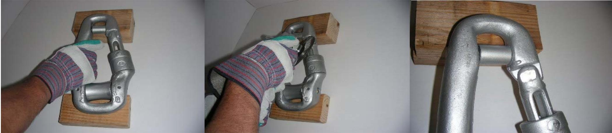
**STEP 3:** Grasp & flip the Ring over so that the Push-Button is now facing downwards. Repeat Step 2 on this side of the Ring.
