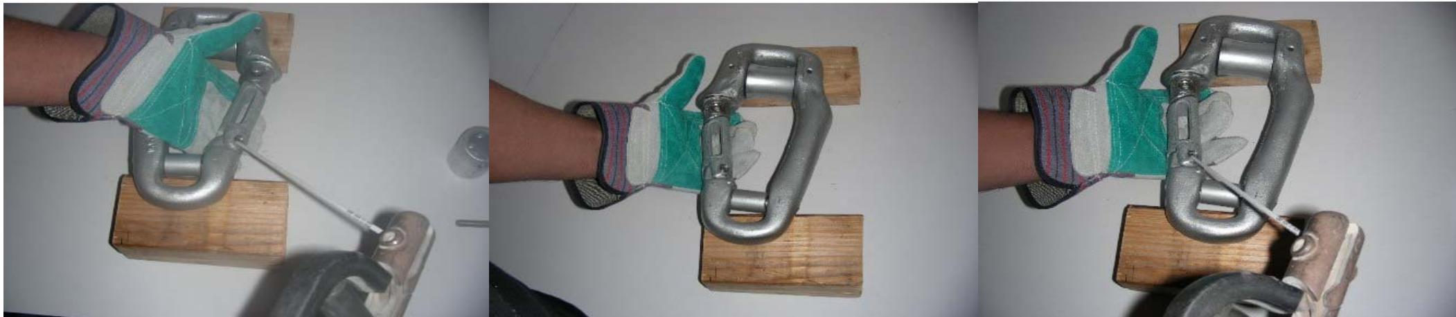
**STEP 6:** Using the stick of special welding rod provided, weld over the pin & hole. Once finished, flip the Ring over & repeat the process on the other side.
