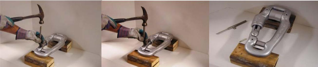
**STEP 2:** Place the narrow end of the smaller Tool Set into one of the holes for pin. Hammer down on the opposite end of the Tool Set until the pin falls down & out of the Ring.
