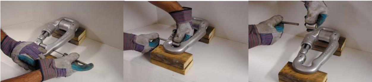
**STEP 3:** Place the thin end of the Tool Set into the hole for shaft & push. Grab hold of roller & end of shaft now sticking out. Pull shaft out of hole, freeing both shaft & Roller #2.
