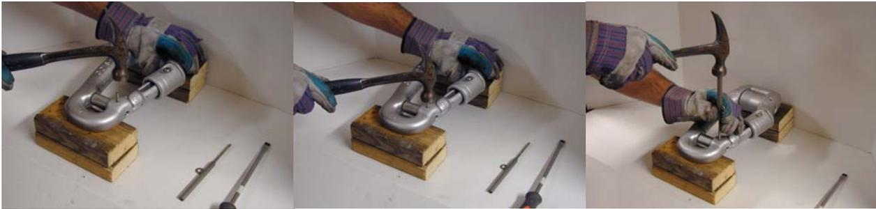
**STEP 6:** Insert new pin into the hole for pin. Hammer the pin down until it is flush with the Ring. Place the narrow end of the smaller Tool Set on the pin. Lightly hammer down on the opposite end of the Tool Set so that the pin sits just below the level of the Ring. The pin's depth should be equal on both side sof the Ring.
