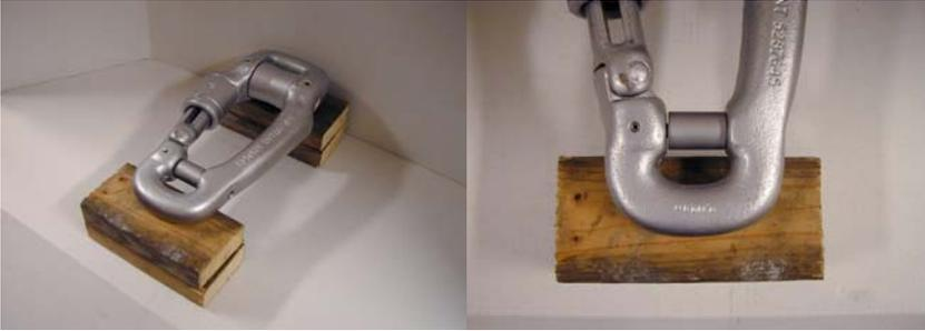
**STEP 1:** Clear a stable area. Using solid materials create 2 points of elevation. Place the Ring on top of these 2 points with the Push-Button facing downwards. Make sure the Roller #2 hole for pin is free of the point of elevation so that the pin may be hammered out later.
