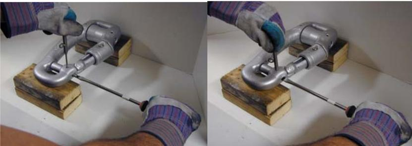
**STEP 4:** Flip the Ring over so that the Push-Button is now facing upwards. Hold the new Roller #2 in place & then slide the non-grooved end of the new shaft into the Ring & new Roller #2. Once in, place the smaller Tool Set into the hole for pin & place a flat head screwdriver into the groove end of the new Shaft. Push down on the Tool Set & turn the screwdriver until the holes for pins line up with those on the new Shaft, at which point the Tool Set will slide further in.
