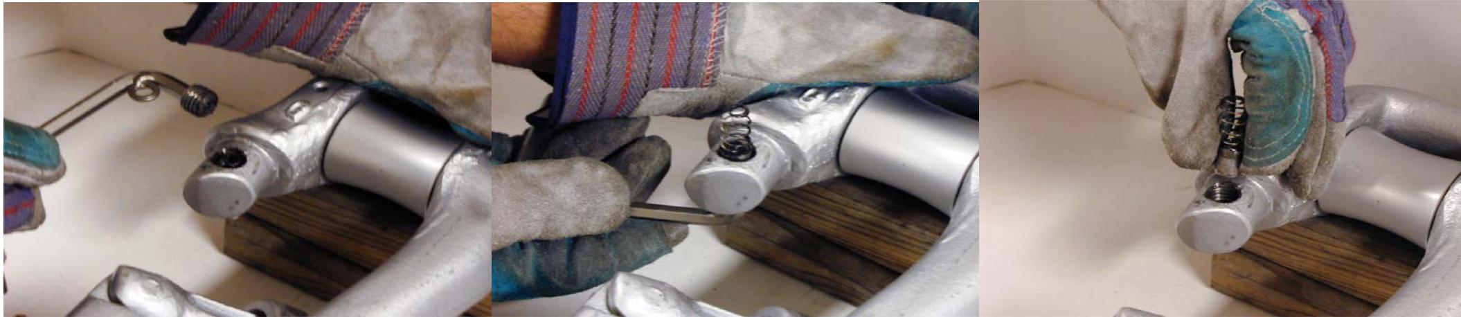
**STEP 3:** Now that the Set-Screw is free, remove it from the end of the Tool Set. Place the same end of the Tool Set on the underside of the Push Button Assembly & push up. Now remove the last two pieces from the Ring.
