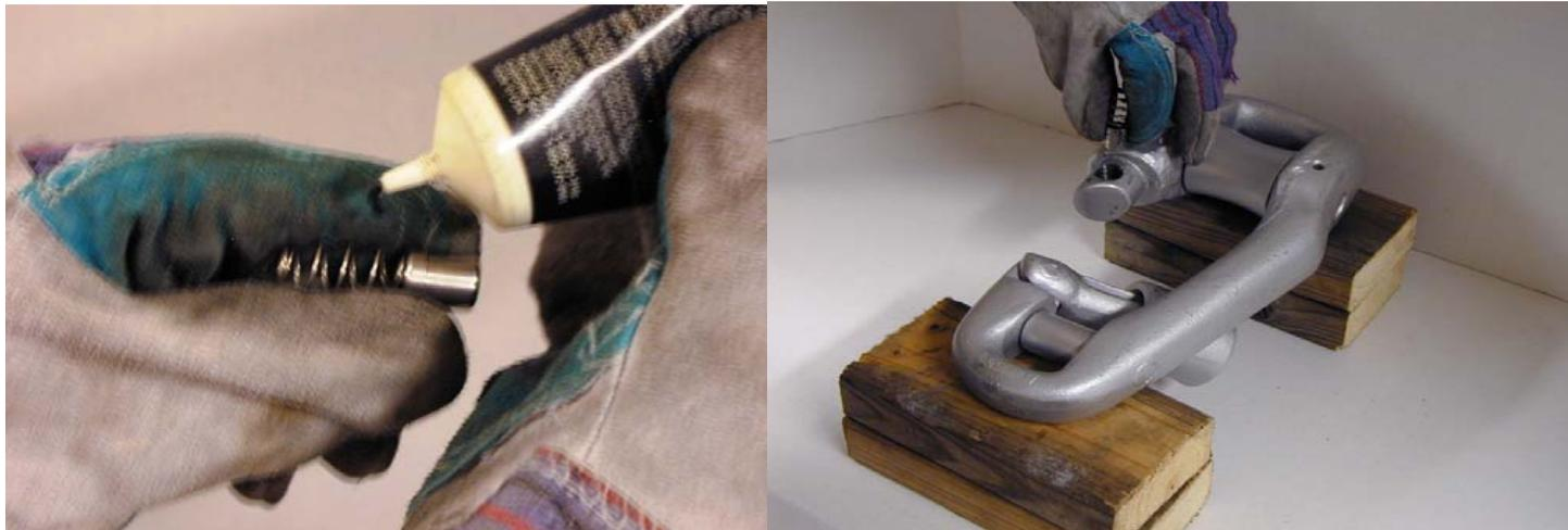
**STEP 4:** Grasp the Push-Button & Spring from the new Push-Button Assembly & place a fair amount oil-type lubricant on the 2 pieces. Now drop the 2 pieces into the whole for the Push-Button Assembly. Be sure to drop the Push-Button piece in first with the narrow end pointing downwards.
