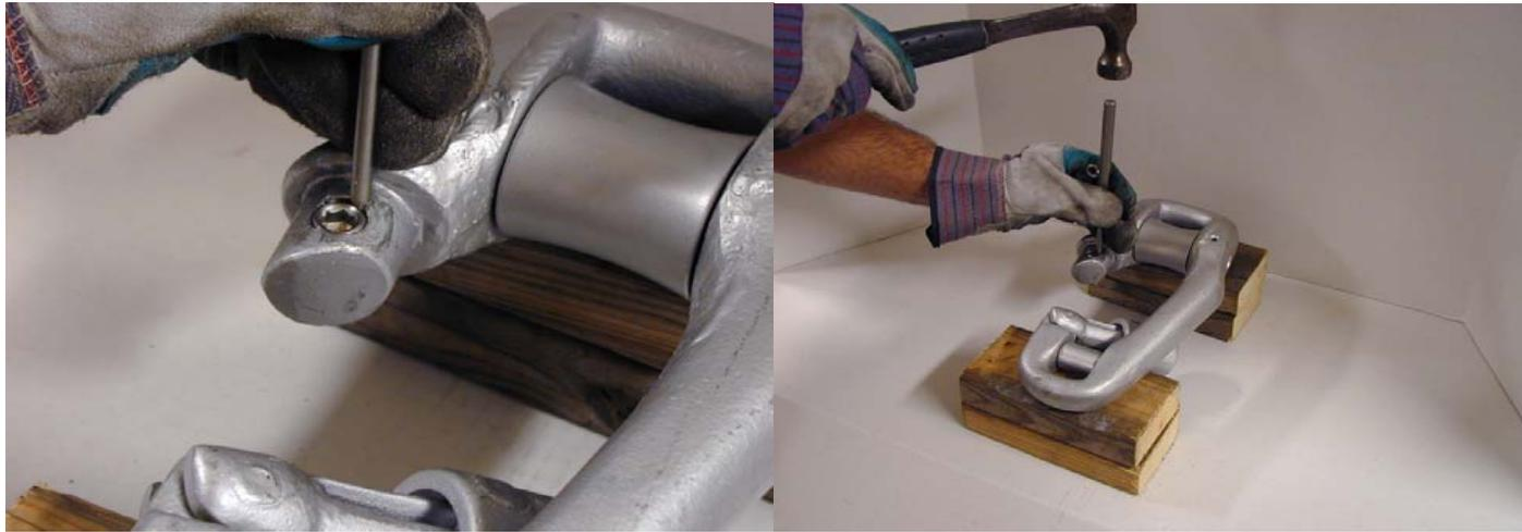
**STEP 6:** Now take a center punch & place the sharp end between the Set Screw & Ring. Using medium strength hammer down on the fat end of the center punch to create a small divot. Find another spot between the Set Screw & Ring, & repeat process.
