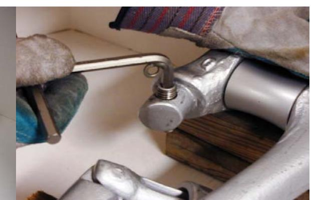
**STEP 2:** Place the curved short end of the Tool Set into the back end of the Push-Button Assembly, called the Set-Screw. Turn the Tool Set counterclockwise until the piece is free of the Ring.
