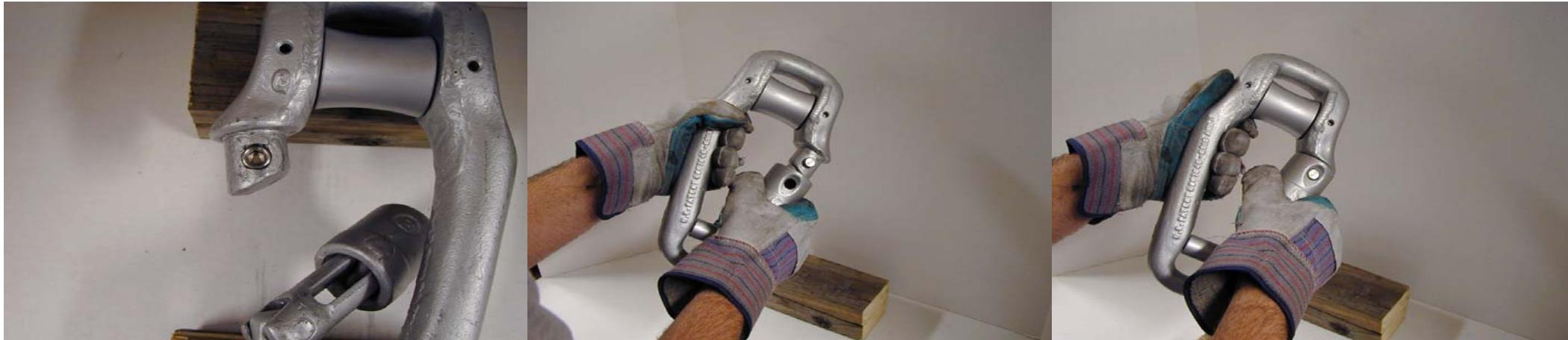
**STEP 6:** Now that the Push-Button Assembly is in place, flip the ring over to close & open the Sleeve Assembly. Perform this test a few times to make sure the Push-Button is not making it difficult to close the Sleeve Assembly & that it is also stopping the Sleeve Assembly from opening when secure. If either of these situations are occurring, adjust the Set Screw up or down until the testing works properly.
