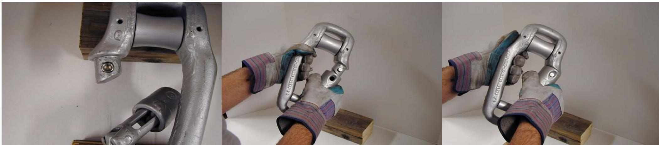
**STEP 6:** Now that the Push-Button Assembly is in place, flip the ring over to close & open the Sleeve Assembly. Perform this test a few times to make sure the Push-Button is not making it difficult to close the Sleeve Assembly & that it is also stopping the Sleeve Assembly from opening when secure. If either of these situations are occurring, adjust the Set Screw up or down until the testing works properly.
