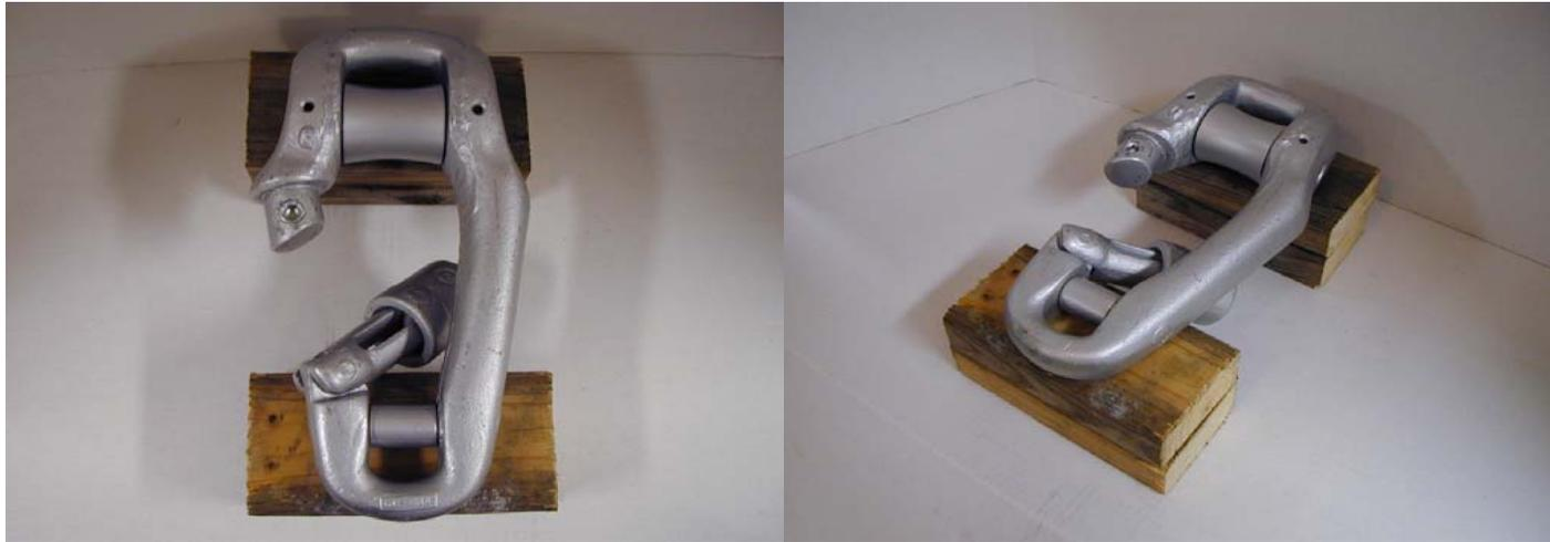
**STEP 1:** Clear a stable area. Using solid materials create 2 points of elevation. Place the Ring on top of these 2 points with the Sleeve Assembly open & Push-Button facing downwards. Make sure the Push-Button is free of the point of elevation so that it may be pushed up & out later.
