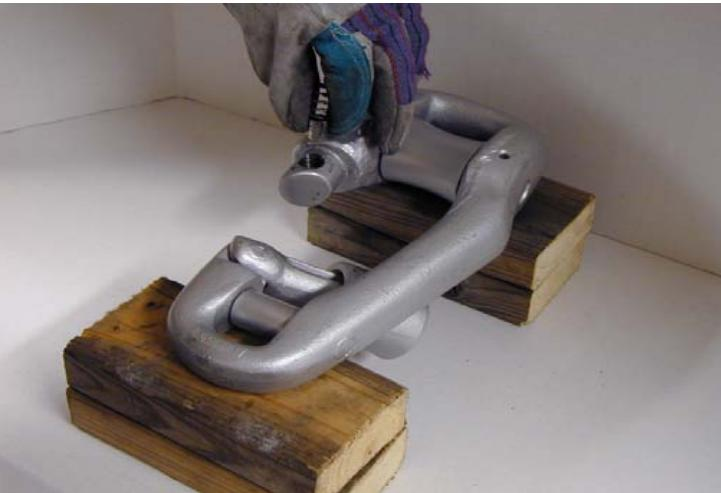
**STEP 4:** Grasp the Push-Button & Spring from the new Push-Button Assembly & place a fair amount oil-type lubricant on the 2 pieces. Now drop the 2 pieces into the hole for the Push-Button Assembly. Be sure to drop the Push-Button piece in first with the narrow end pointing downwards.
