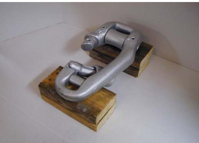
**STEP 1:** Clear a stable area. Using solid materials create 2 points of elevation. Place the Ring on top of these 2 points with the Sleeve Assembly open & Push-Button facing downwards. Make sure the Push-Button is free of the point of elevation so that it may be pushed up & out later.
