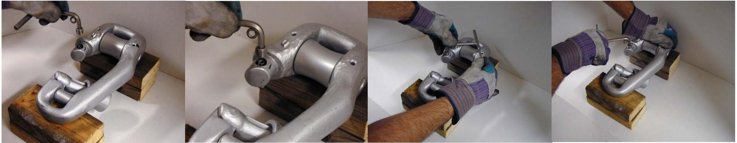
**STEP 5:** Place the Set-Screw on the curved short end of the Tool Set. Now place the Set Screw in the whole for the Push-Button & turn the Tool Set clockwise until the Set-Screw sits flush with the rest of the Ring.
