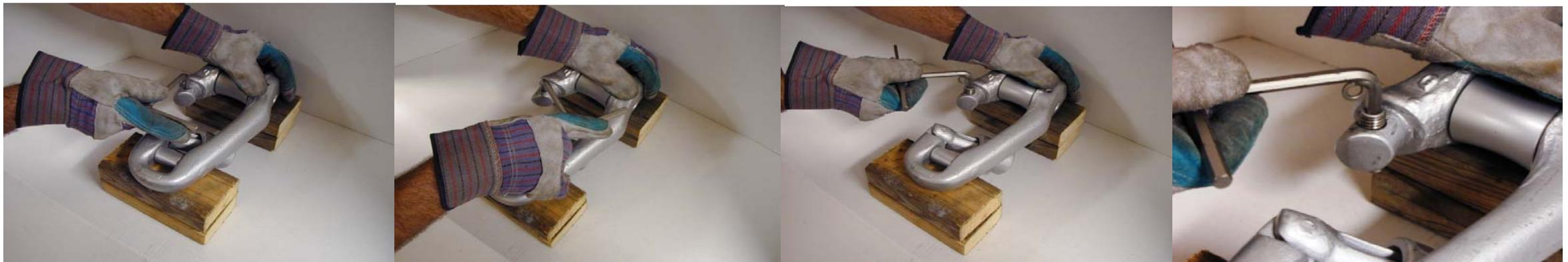
**STEP 2:** Place the curved short end of the Tool Set into the back end of the Push-Button Assembly, called the Set-Screw. Turn the Tool Set counterclockwise until the piece is free of the Ring.
