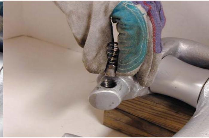
**STEP 3:** Now that the Set-Screw is free, remove it from the end of the Tool Set. Place the same end of the Tool Set on the underside of the Push Button Assembly & push up. Now remove the last two pieces from the Ring.
